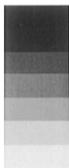
Figure 8. Grayscale ruler, for comparison with figures. Each step corresponds to 1.2 V. The scale is compressed at the ends, making the last three steps to white (−6 V) not visible. The top of the scale (black) corresponds to +6 V.
