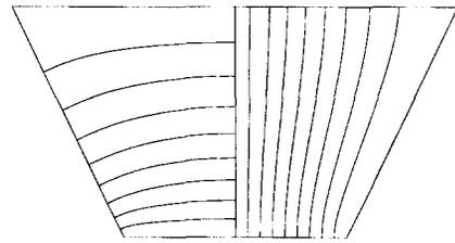
Fig. 3. Equipotentials and flow lines for computed resistance.
