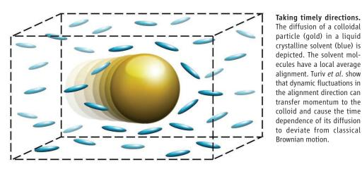
new example of "anomalous diffusion" of colloids that involves a liquid crystal (LC), a liquid-like phase that has long-range orientational ordering. Fluctuations in the solventmolecule orientations cause MSDs of colloids to grow nonlinearly with time.
