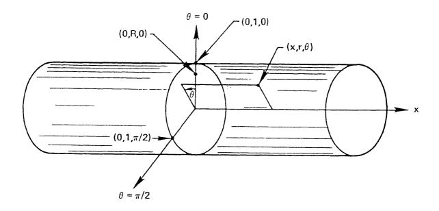
Figure 1. Coordinate System for Cylindrical Cell.
