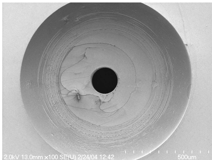
Figure 1. Scanning electron micrograph of an aperture with a diameter of 150 \mu\text{m} , etched inside a 1 \text{ mm} wide recess. The substrate used was a double side polished wafer with a thickness of 380 \mu\text{m} . Both recess and aperture were etched using reactive ion etching with cyclic etch and passivation steps (Bosch process). The area inside the recess has been thinned down to match the diameter of the aperture. The additional circular features visible are steps that arise due to the concave bottom profile created during the recess etch.
