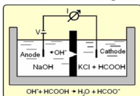
Sodium hydroxide etches along the damage track until breakthrough occurs and the etching is stopped.
