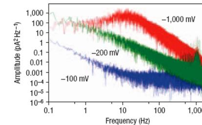
Power spectra of the ion current recordings above. The peak between 10 Hz and 20 Hz for the -1,000 mV time series corresponds to oscillations of that frequency, which can be clearly seen from the time series.
