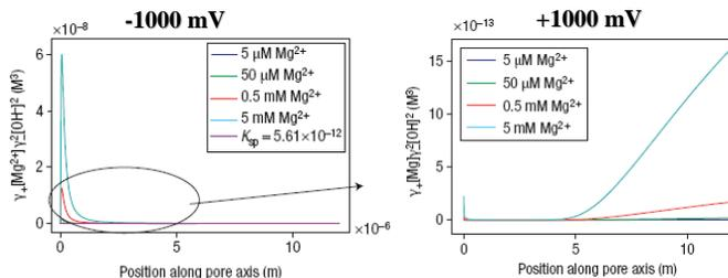
Theoretical results from the one-dimensional Poisson-Nernst-Planck model mapping the products of the magnesium and hydroxide activities for -1,000 mV (left), +1,000 mV (right), along the pore axis. The modeling confirms that the ionic concentrations in the pore are very different for the two voltage polarities, allowing the nanoprecipitates to form for negative voltages.
