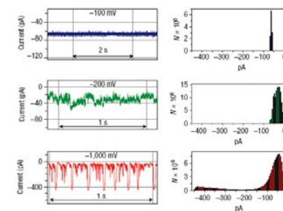
Ion current time series along with current histograms for various applied voltages as indicated, with 0.1 M KCl, 0.2 mM CaCl<sub>2</sub> and 5 mM PBS.
