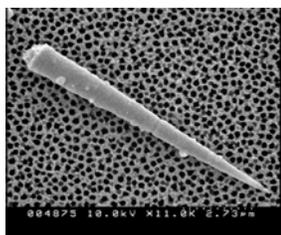
A gold electrodeless deposition "negative" of a conical PET nanopore. (Univ. of Florida)
