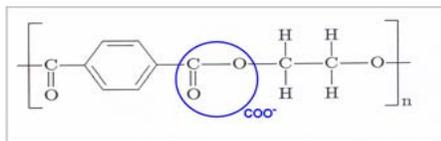
Etching PET with NaOH produces carboxyl groups on the polymer surface. Surface density of these groups is estimated at ~1.5 per nm<sup>2</sup>.
