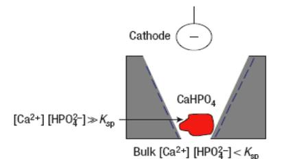
When the negatively biased electrode (cathode) is at the larger opening of a conical nanopore, cations will move from the narrow opening towards the larger opening of the cone. The activities of Ca<sup>2+</sup> and HPO<sub>4</sub><sup>2-</sup> ions inside the nanopore then rise above the solubility product K<sub>sp</sub> of CaHPO<sub>4</sub>, allowing nanoprecipitation to occur.
