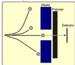
A high energy single heavy ion creates a damage track through the polymer film.
