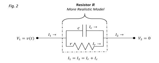
The circuit in Fig. 2 is described by the circuit equations
