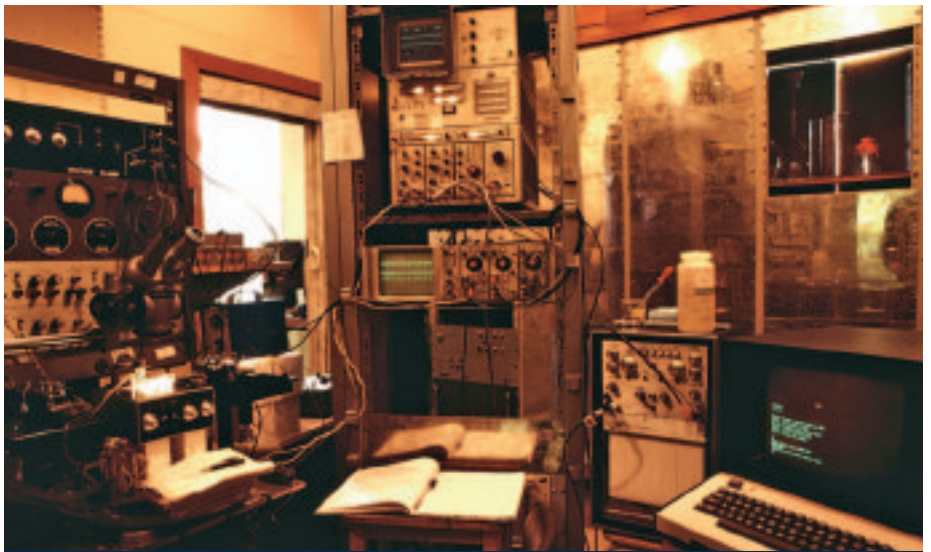
The inner sanctum of Otto Hutter's lab. Anne Warner's storage oscilloscope is in the centre. The high-speed chart recorder just to the right provided a complete history of each cell. Baseline drifts, etc. become obvious on a slower time scale. One day there was a thunderstorm; each bolt of lightning left a dramatic impression on the current noise records!
