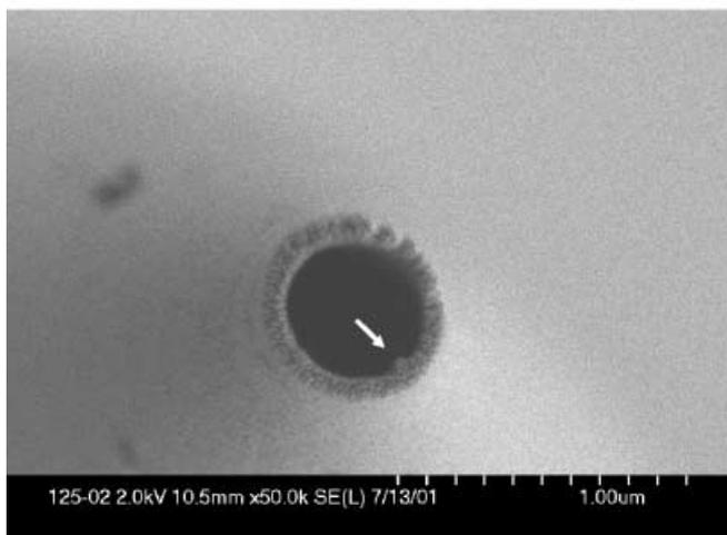
**Fig. 2** **a** Light micrograph depicting tip taper of pipettes used. **b** Scanning electron micrograph looking into the pipette bore. The arrow shows the location of internal filament
