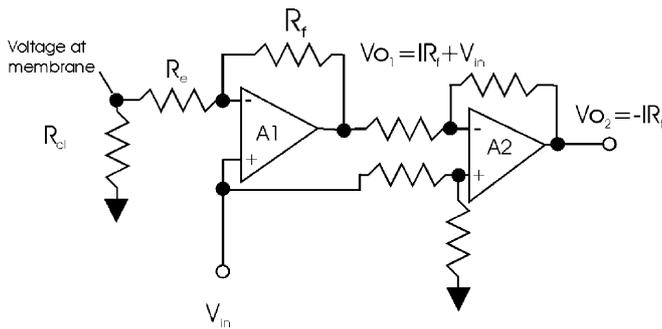
**Fig. 1** Circuit diagram for electroporation apparatus [ $R_f$  feedback resistance,  $R_e$  electrode resistance,  $R_{cl}$  cleft resistance,  $V_{in}$  command voltage to be applied to the pipette interior,  $V_{O1}$  output voltage of the current-to-voltage converter (A1),  $V_{O2}$  output of the differential amplifier (A2)]
